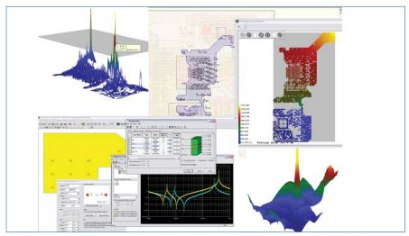
HyperLynx PI includes pre- and post-layout power integrity analysis, such as DC drop analysis, AC decoupling analysis, plane noise analysis, and model extraction.
